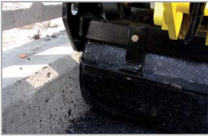
New: reduced overhang and improved wall clearance.
