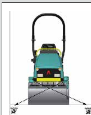
4 large tie down points for safe fixing onto trailer / truck
