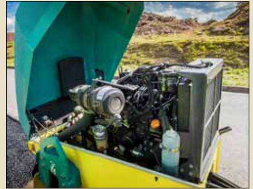
Best service access due to large engine hood
