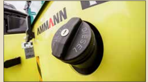
Lockable diesel-tank standard
