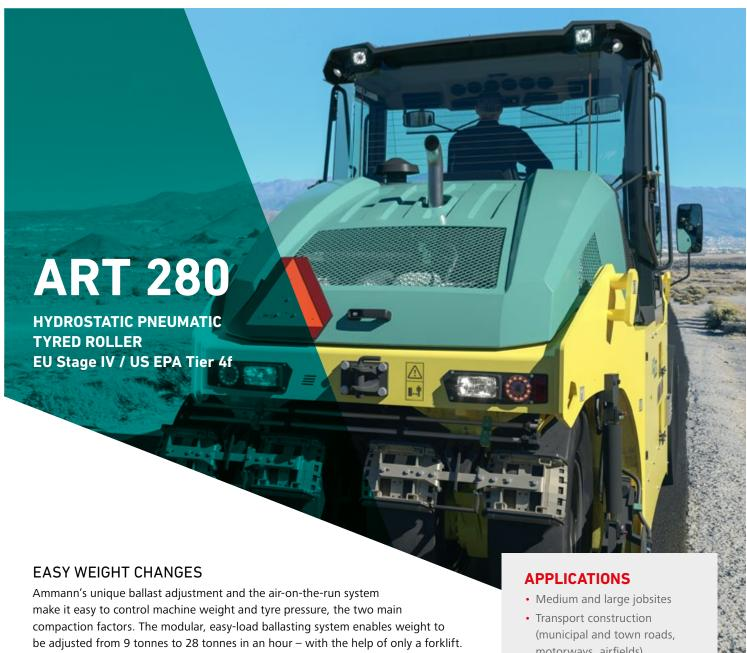
Brand new cab reduces sound and boosts operator comfort and safety. Improved serviceability keeps crews productive and maintenance costs to a minimum. The roller is powered by the latest EU Stage IV / US EPA Tier 4f engine from Deutz with EGR, DOC and SCR technology.
