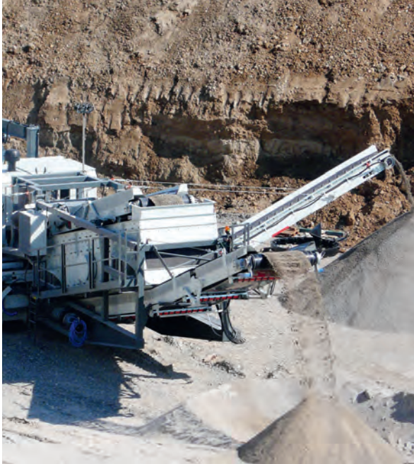
3-Deck Siebmaschine 1800 x 6000 mm
